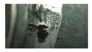
**Extractor marks** - After a semi-automatic pistol has been fired, an extractor pulls the cartridge from the chamber and ejects it from the pistol.
