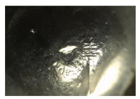
**Firing pin impressions** - When a firearm's trigger is pulled, the firing pin will move forward striking the primer cup located at the rear center of the cartridge.
