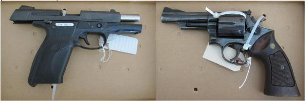
The use of zip ties in the position(s) pictured will allow lab staff to see that the weapon is unloaded in addition to securing it to the box. The use of commercially available gun boxes with a window is **required** for all handgun submissions.
