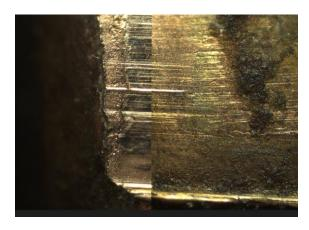
The photo on the left shows the split screen image the scientist sees using the comparison microscope. The right side of the photo shows the test bullet fired from the suspect's firearm into the water tank and the left side, the bullet recovered from the crime scene. The marks or striations on the evidence bullet were identified as being made by the suspect's firearm.
