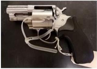
The use of zip ties in the position(s) pictured will allow lab staff to see that the weapon is unloaded in addition to securing it to the box. The use of commercially available gun boxes with a window is encouraged. This will help expedite the verification process by removing the need for the box to be opened in the evidence receiving area.
