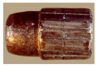
The impressions of lands and grooves are transferred to the bullet when it is fired.
