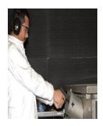
The first step in the **Comparison Process** is to test fire the firearm into a water tank in the lab.
