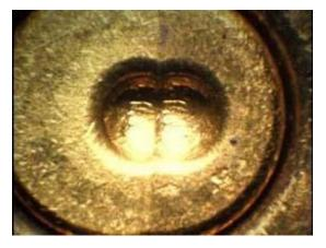
**Firing pin impressions** - When a firearm's trigger is pulled, the firing pin will move forward striking the primer cup located at the rear center of the cartridge.
