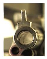
Inside the barrels of handguns and rifles are spiral impressions called rifling. The raised portions of the rifling are known as lands and the recessed portions are known as grooves. When a weapon is fired, these lands and grooves cut into the bullet, putting spin on it as it travels through the barrel of a firearm. Because bullets have an oblong shape, spin is necessary for accurate flight.
