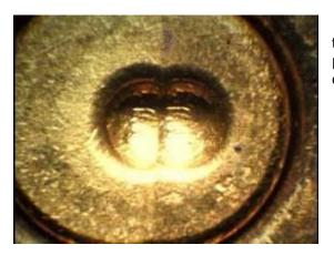
**Firing pin impressions** - When a weapon's trigger is pulled, the firing pin is forced into the primer cup located at the rear center of the cartridge.
