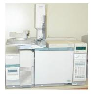
The extracted sample is analyzed on a Gas Chromatograph Mass Spectrometer (GCMS).
